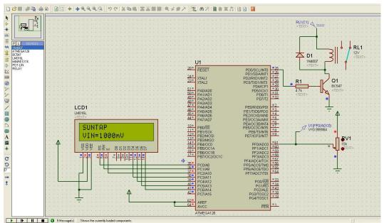
Fig5. Simulation setup for Battery charging switching diagram
