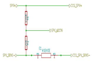
Fig.3.Circuit diagram of sensing of battery voltage
