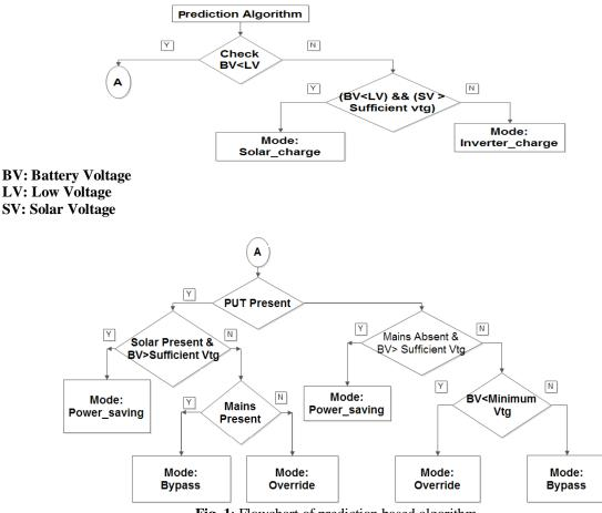
Fig. 1: Flowchart of prediction based algorithm
